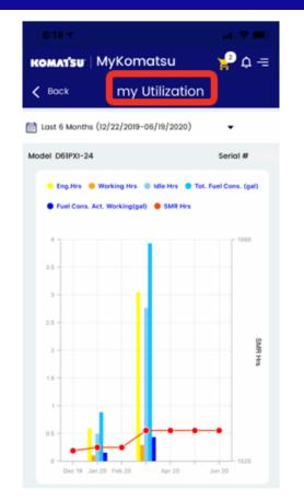
Click on my Utilization tab on top to gain instant access to Komtrax Utilization data
